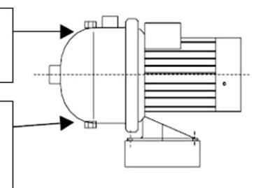
Air and CO2 inlet: connect  $\phi$ 12 high pressure PU windpipe with quick-acting.
