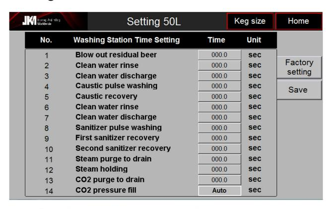
In this picture, the customer types according to their own keg, choosing the appropriate cleaning program, press the corresponding button, You choose the bucket will be off. Click the time setting, can be revised based on the default time, we provide open parameter setting function, convenient to customers according to their own actual situation to adjust.
