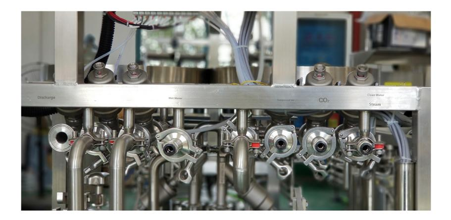
The connector from left to right is Discharge, Hot water, CO2, Compressed air, Sterile steam/ Clean water(RO water)
