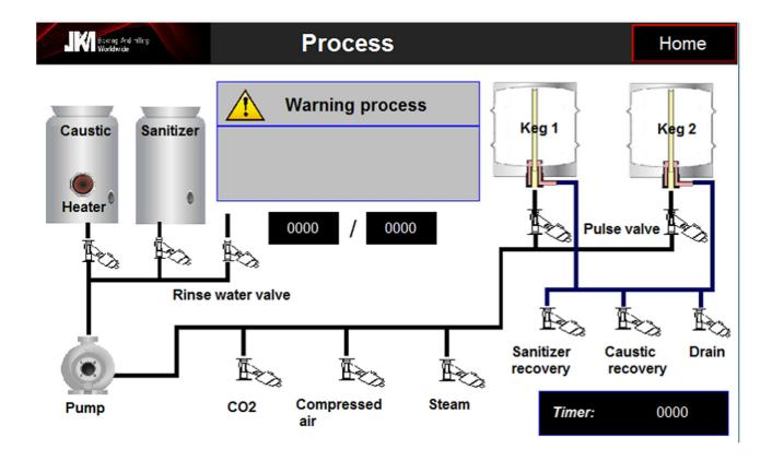
The operator can see all parts of the machine in this screen, when you touch the start button on the stainless surface,
