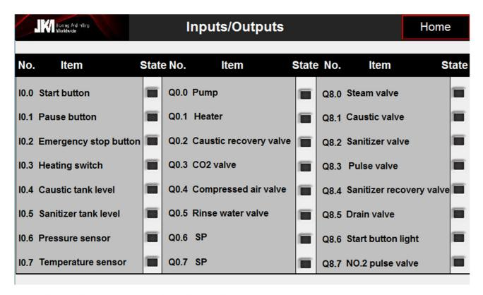
This picture is used to monitor the various components or instrument at present state of the signal Such as machine external components damaged, can be checked by the interface.
